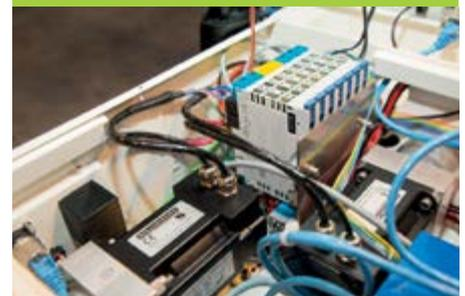
Even in the confined interior of the AGV PackMan 200, there is space for the vibration-proof S-DIAS system with motion control and Safety, as well as two AKM low-voltage DC servo motors.
