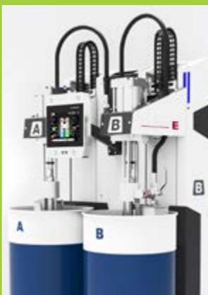
The dosing system Top 5000P for LSR dosing and fluid silicon processing does not require a control cabinet thanks to the compactness of the S-DIAS control and I/O system. A unique user experience is provided by the “floating” HMI, which can be intuitively operated and flexibly placed.
